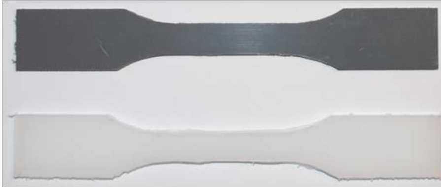
Figure F.2 The visual appearance of neat PVC (top) and PP (bottom)
